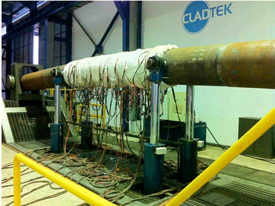
FIGURE 3: Photograph of Test Pipe on Test Rig with Heating and Instrumentation
