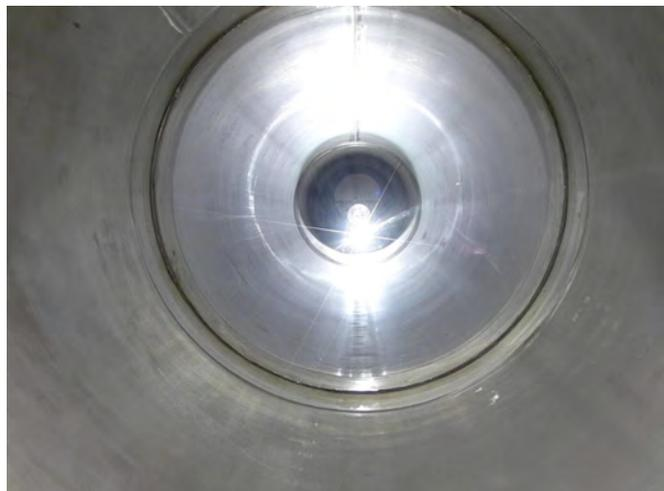
**FIGURE 6 - NPS 24 Lined Pipe - No Wrinkles after +/-0.4% Strain (Ambient)**
