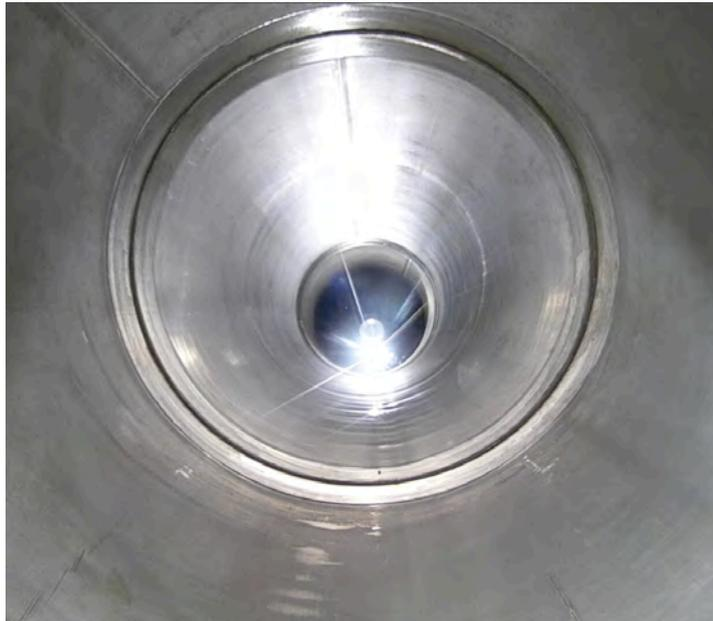
**FIGURE 9: NPS 24 Lined Pipe - Wrinkles at -1.0% strain 110°C with ZERO overpressure**
