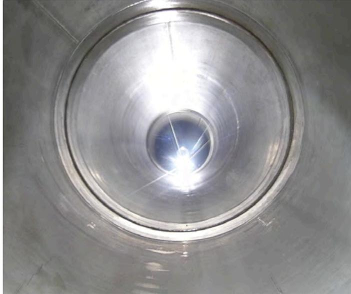
**FIGURE 8: NPS 24 Lined Pipe - No wrinkles at -0.80% strain, 110°C and 20barg**
